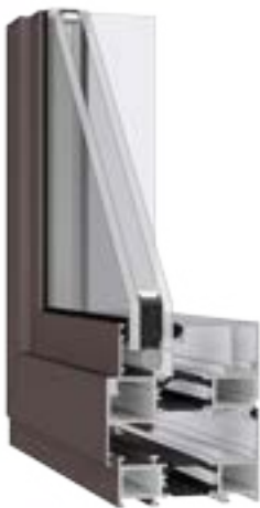
G201 A Project Out window, also know as an Awning with an AAMA rating of AW 100, and a U-Value of 0.363.
