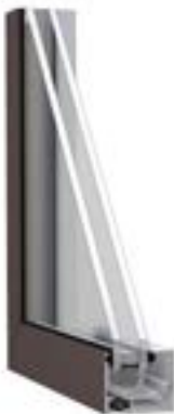
G741 A Fixed window with an AAMA rating of AW 70, and a U-Value of 0.293.
