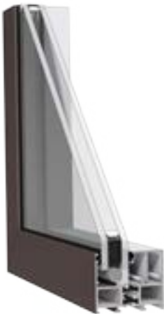
G141 A Fixed window with an AAMA rating of AW70, and a U-Value of 0.314.
