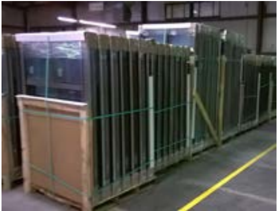
Example of palletizing windows for easier loading and unloading of trucks.
