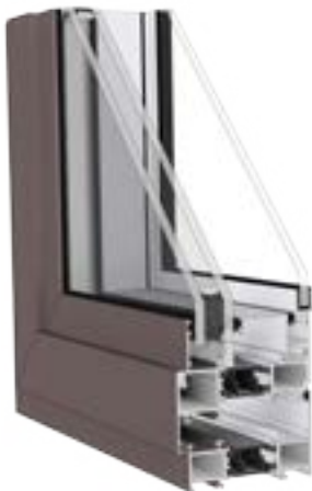
G401 A Project Out Awning window with an AAMA rating of AW 100, and a U-Value of 0.281.
