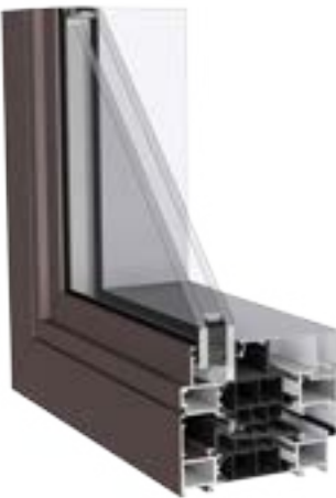
G5T1 A Dual Action Casement Inswing Left with an AAMA rating of AW 60, and a U-Value of 0.16.
