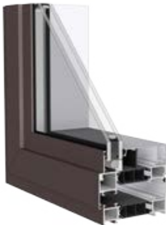
G561 A Casement Inswing Left with an AAMA rating of AW 80, and a U-Value of 0.176.
