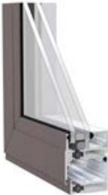
G751 A Casement Outswing Left window with an AAMA rating of AW100, and a U-Value of 0.384.
