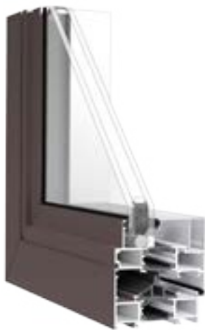
G211 A Project In/Hopper window with an AAMA rating of AW 100, and a U-Value of 0.375.
